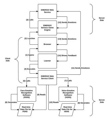
Figure 1. Data flow of the software system architecture.
